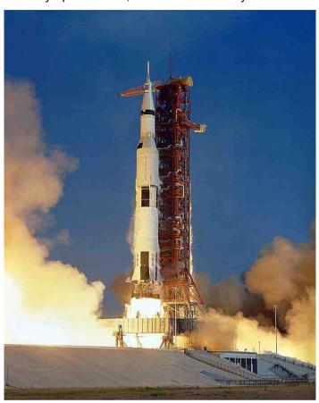
[Above] This Saturn V vehicle lifted off at a total mass of some 3.000 tonnes!
